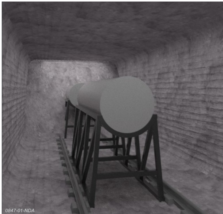
Figure A10 Illustration of a Geological Disposal Facility High Level Waste disposal tunnel in evaporite rock (Nuclear Decommissioning Authority, UK)
